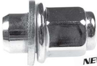
611-214 Chrome NEW! Thread Hex Size Length Seat M12-1.5 21mm 42mm 18.43mm dia. x 12.31 lg.
