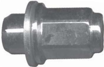
611-167 Chrome Thread Hex Size Length Seat M12-1.5 21mm 47mm 18.5 dia. x 12.0 lg.
